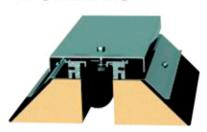
The L Series is a center plate system designed for roof expansion joint applications. It has a centering device to provide mechanical attachment of the metal center plate to metal frames that allows plus and minus 50-100% thermal and seismic movement in nominal expansion joint gaps of 1 to 18 inches. It has an internal moisture barrier that can be directed to drains or exterior wall covers to evacuate water.
