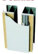
The G Series are snap-on or clip-in cover systems designed for wall and ceiling expansion joint applications. The snap-on device has a hidden fastener to provide mechanical attachment of the metal cover plate to the substrate. The clip-in cover systems are attached using stainless steel internal fasteners. These allow plus and minus 25-50% thermal movement in nominal expansion joint gaps of 1 to 2 inches.
